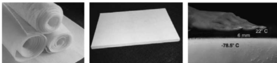
Figure 46. Flexible aerogel blankets and solid aerogel boards: (a) aerogel blankets [147], (b) aerogel panel [148], and (c) super-insulating aerogel blanket [147].
