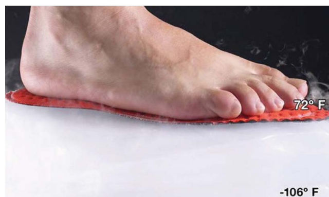
Figure 47. Difference between the temperature below and above the aerogel-insulated footwear [149].
