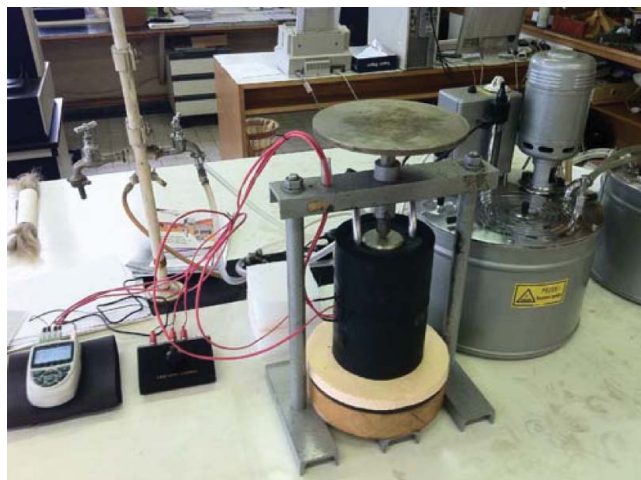
Figure 22. Device for measuring thermal conductivity [55].
